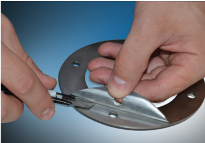
Surface Bonded Laminated Shims must be adjusted using a tool.
